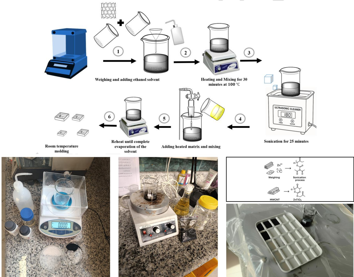
Fig. 4. Experimental procedure for laboratory-scale nanocomposite fabrication
